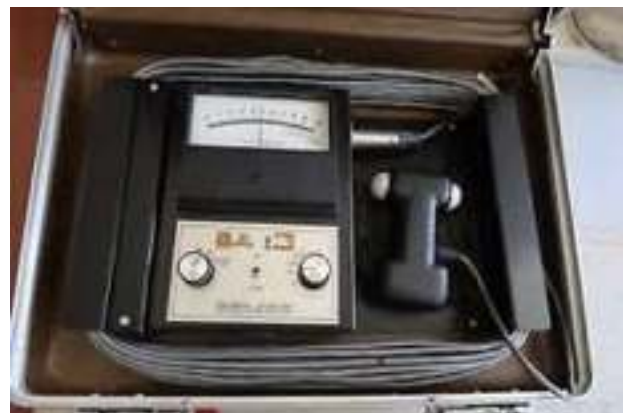
Figure 6: Protomatic light photometer Source: ebay.com
