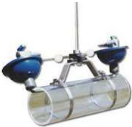
Figure 7: Van Dorn Bottle Sampler Source: ecoenvironmental.com
