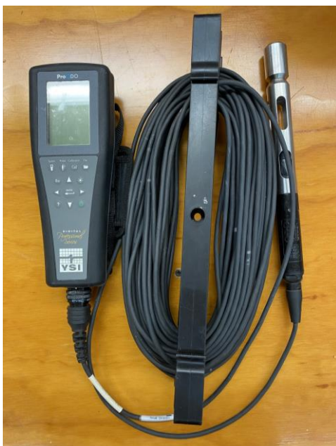
Figure 3: YSI probe used to measure temperature and dissolved oxygen.
