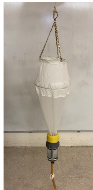
Figure 7: 80 \mu\text{m} net used to collect plankton
